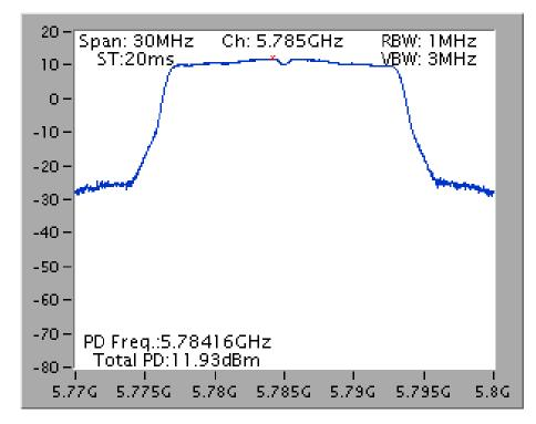
Power Density Plot on Configuration IEEE 802.11a / Ant. 1 + Ant. 2 / 5785 MHz
