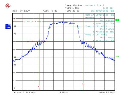
26dB Bandwidth and 99% Occupied Bandwidth Plot on Configuration IEEE 802.11a / Chain 1 + Chain 2 / 5745 MHz
