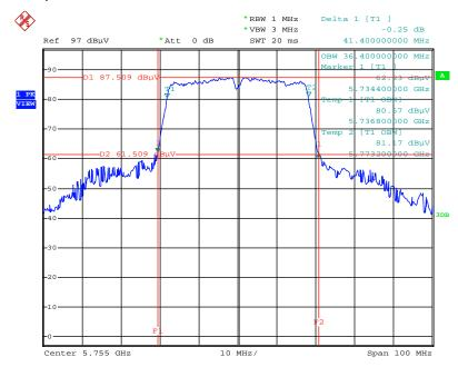
26dB Bandwidth and 99% Occupied Bandwidth Plot on Configuration IEEE 802.11ac MCS0/Nss1 VHT40 / Chain 1 + Chain 2 / 5755 MHz
