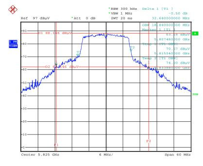
26dB Bandwidth and 99% Occupied Bandwidth Plot on Configuration IEEE 802.11a / Chain 1 + Chain 2 / 5825 MHz
