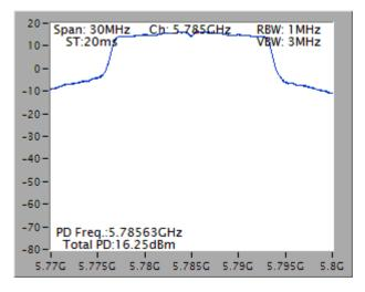
Power Density Plot on Configuration IEEE 802.11a / Chain 1 + Chain 2 / 5785 MHz
