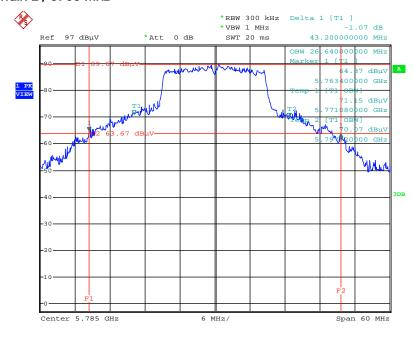
26dB Bandwidth and 99% Occupied Bandwidth Plot on Configuration IEEE 802.11ac MCS0/Nss1 VHT20 / Chain 1 + Chain 2 / 5785 MHz
