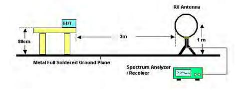
For Radiated Emissions: 30MHz~1GHz
