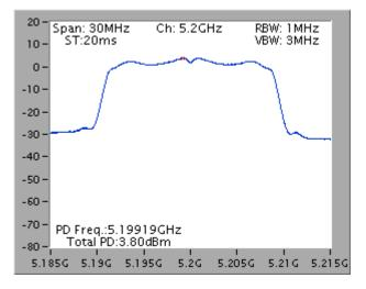
Power Density Plot on Configuration IEEE 802.11n MCS0 20MHz / Ant. 1 + Ant. 3 / 5200 MHz
