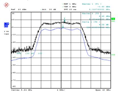
Peak Excursion Plot on Configuration IEEE 802.11a / Ant. 1 + Ant. 3 / 64QAM(48Mbps) / 5240 MHz
