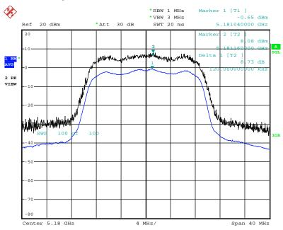
Peak Excursion Plot on Configuration IEEE 802.11n 20MHz / Ant. 1 + Ant. 3 / 16QAM(MCS3) / 5180 MHz
