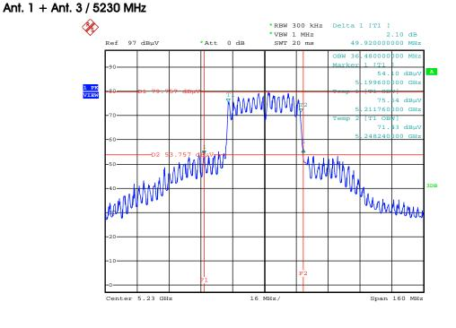
26dB Bandwidth and 99% Occupied Bandwidth Plot on Configuration IEEE 802.11n MCS0 40MHz /
