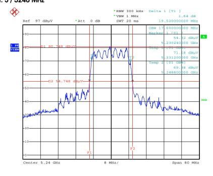
26dB Bandwidth and 99% Occupied Bandwidth Plot on Configuration IEEE 802.11n MCS0 20MHz / Ant. 1 + Ant. 3 / 5240 MHz
