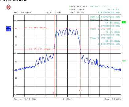
26dB Bandwidth and 99% Occupied Bandwidth Plot on Configuration IEEE 802.11n MCS0 20MHz / Ant. 1 + Ant. 3 / 5180 MHz
