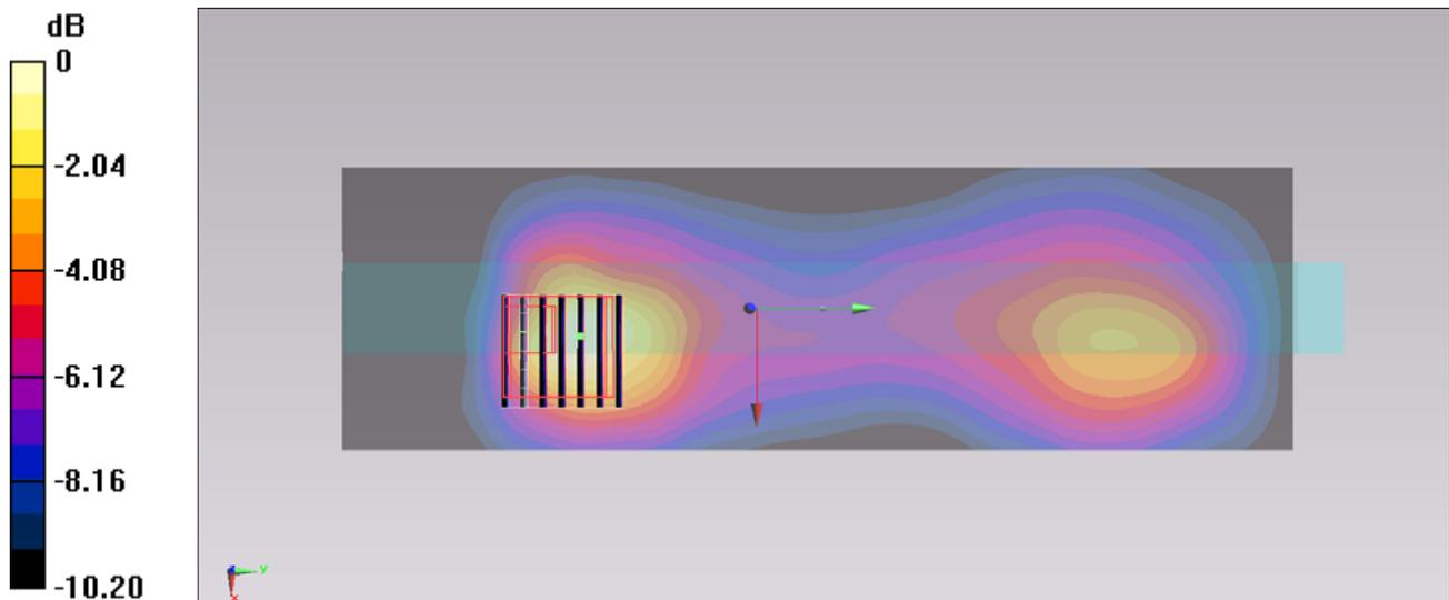
0 dB =  $2.76 \text{ W/kg} = 4.41 \text{ dBW/kg}$
