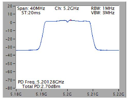
Power Density Plot on Configuration IEEE 802.11ac MCS0/Nss1 40MHz / Chain 1 + Chain 2 + Chain 3 / 5230~MHz
