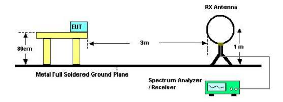
For Radiated Emissions: 30MHz~1GHz
