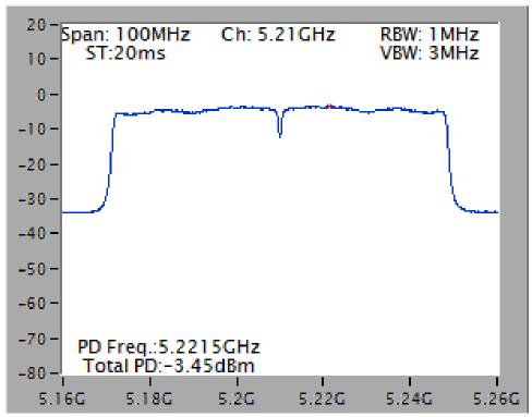
Power Density Plot on Configuration IEEE 802.11a / Chain 1 + Chain 2 + Chain 3 / 5200 MHz
