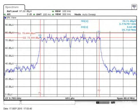
6 dB Bandwidth Plot on Configuration IEEE 802.11ac MCS0/Nss1 VHT80 / Chain 4 + Chain 5 + Chain 6 / 5775 MHz
