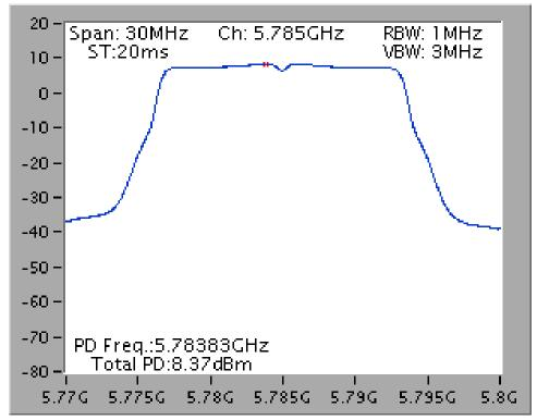
Power Density Plot on Configuration IEEE 802.11ac MCS0/Nss1 VHT20 / Chain 4 + Chain 5 + Chain 6 / 5745 MHz
