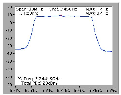
Power Density Plot on Configuration IEEE 802.11ac MCS0/Nss1 VHT40 / Chain 4 + Chain 5 + Chain 6 / 5755 MHz
