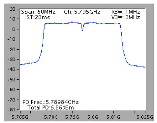
Power Density Plot on Configuration IEEE 802.11ac MCS0/Nss1 VHT80 / Chain 4 + Chain 5 + Chain 6 / 5775 MHz
