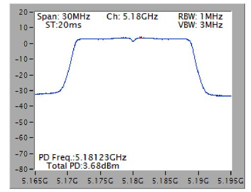
Power Density Plot on Configuration IEEE 802.11n MCS8 HT20 / Ant 3 + Ant 4 / 5180 MHz
