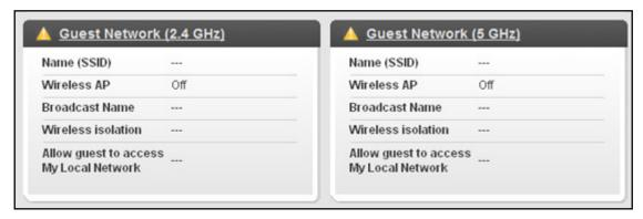
**Name (SSID)**. The 11N wireless network name (SSID) used by the router. The default names are NETGEAR-Guest and NETGEAR-5G-Guest.
