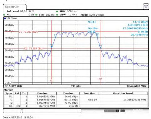
26dB Bandwidth and 99% Occupied Bandwidth Plot on Configuration IEEE 802.11ac MCS0/Nss1 VHT40 / Ant. 1 + Ant. 2 / 5755 MHz
