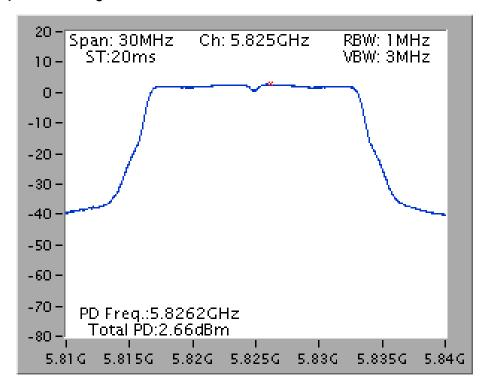
Power Density Plot on Configuration IEEE 802.11n MCS0/Nss1 HT20 / Ant. 1 + Ant. 2 / 5745 MHz
