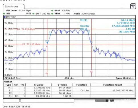
26dB Bandwidth and 99% Occupied Bandwidth Plot on Configuration IEEE 802.11ac MCS0/Nss1 VHT20 / Ant. 1 + Ant. 2 / 5785 MHz
