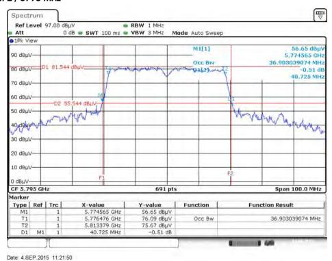
26dB Bandwidth and 99% Occupied Bandwidth Plot on Configuration IEEE 802.11ac MCS0/Nss1 VHT80 / Ant. 1 + Ant. 2 / 5775 MHz
