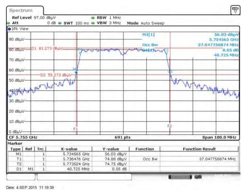
26dB Bandwidth and 99% Occupied Bandwidth Plot on Configuration IEEE 802.11n MCS0 HT40 / Ant. 1
