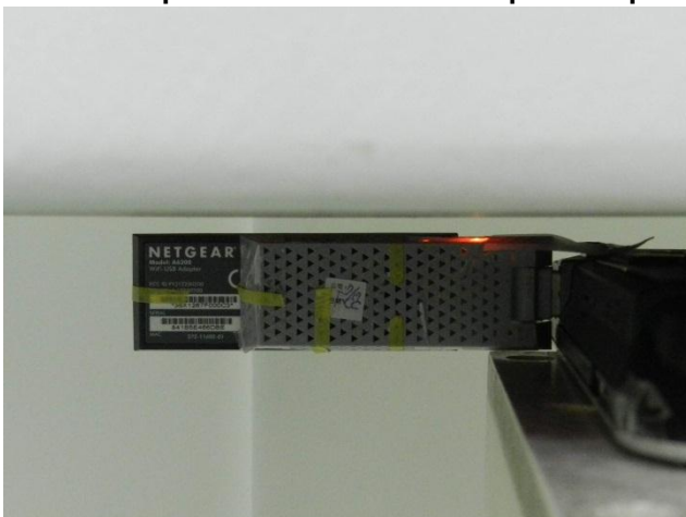
Direct Laptop Plug-in for USB Configuration 3 (Vertical Front with Phantom 5 mm Gap and Flip 180)
