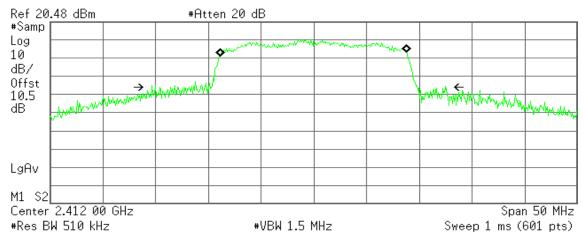
Occupied Bandwidth 17.6297 MHz Occ BW % Pwr 99.00 % x dB -26.00 dB
