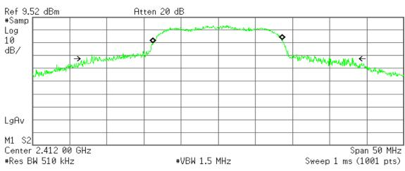
Occupied Bandwidth 17.4041 MHz Occ BW % Pwr 99.00 % x dB -26.00 dB
