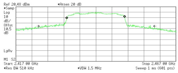
Occupied Bandwidth 17.9537 MHz Occ BW % Pwr 99.00 % x dB -26.00 dB
