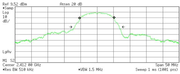
Occupied Bandwidth 10.5037 MHz Occ BW % Pwr 99.00 % x dB -26.00 dB
