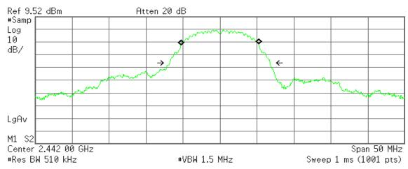
Occupied Bandwidth 10.5002 MHz Occ BW % Pwr 99.00 % x dB -26.00 dB
