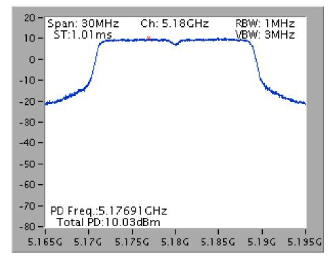
Power Density Plot on Configuration IEEE 802.11n MCS13 HT20 / Chain 1 + Chain 2 / 5180 MHz
