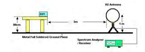
For Radiated Emissions: 30MHz~1GHz
