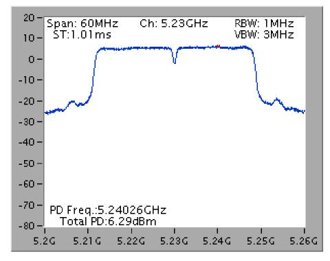
Power Density Plot on Configuration IEEE 802.11n MCS13 HT40 / Chain 1 + Chain 2 / 5230 MHz
