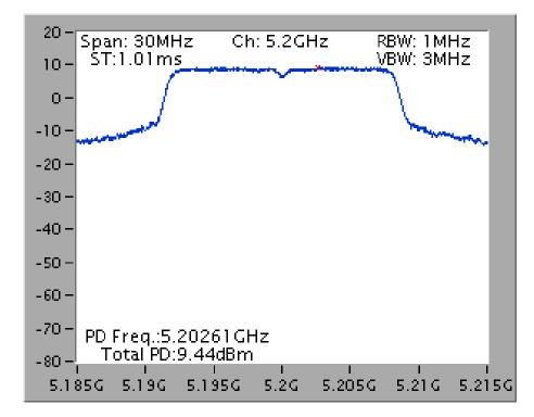
Power Density Plot on Configuration IEEE 802.11a / Chain 1 / 5200 MHz
