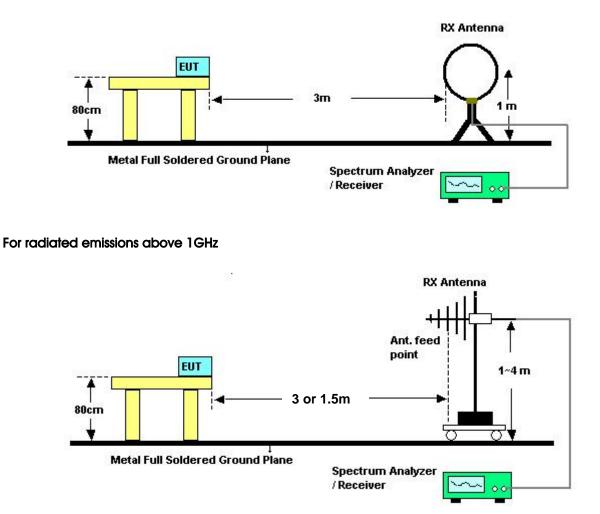
Above 5GHz shall be extrapolated to the specified distance using an extrapolation factor of 20 dB/decade form 3m to 1.5m.
