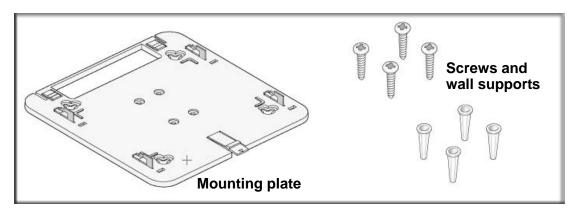
2. Detach the mounting plate from the wireless access point.
