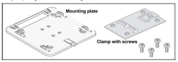
Detach the mounting plate from the wireless access point.
