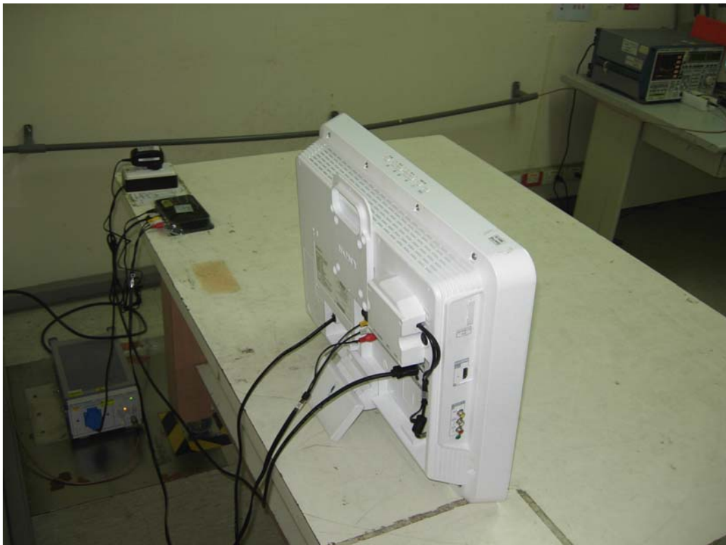
Back View of Conducted Test - (Adapter: MT12-Y120100-A1)
