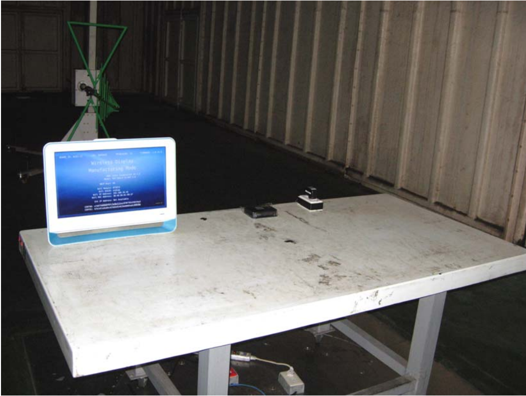
Back View of Radiated Test - (Adapter: T012LF1209)
