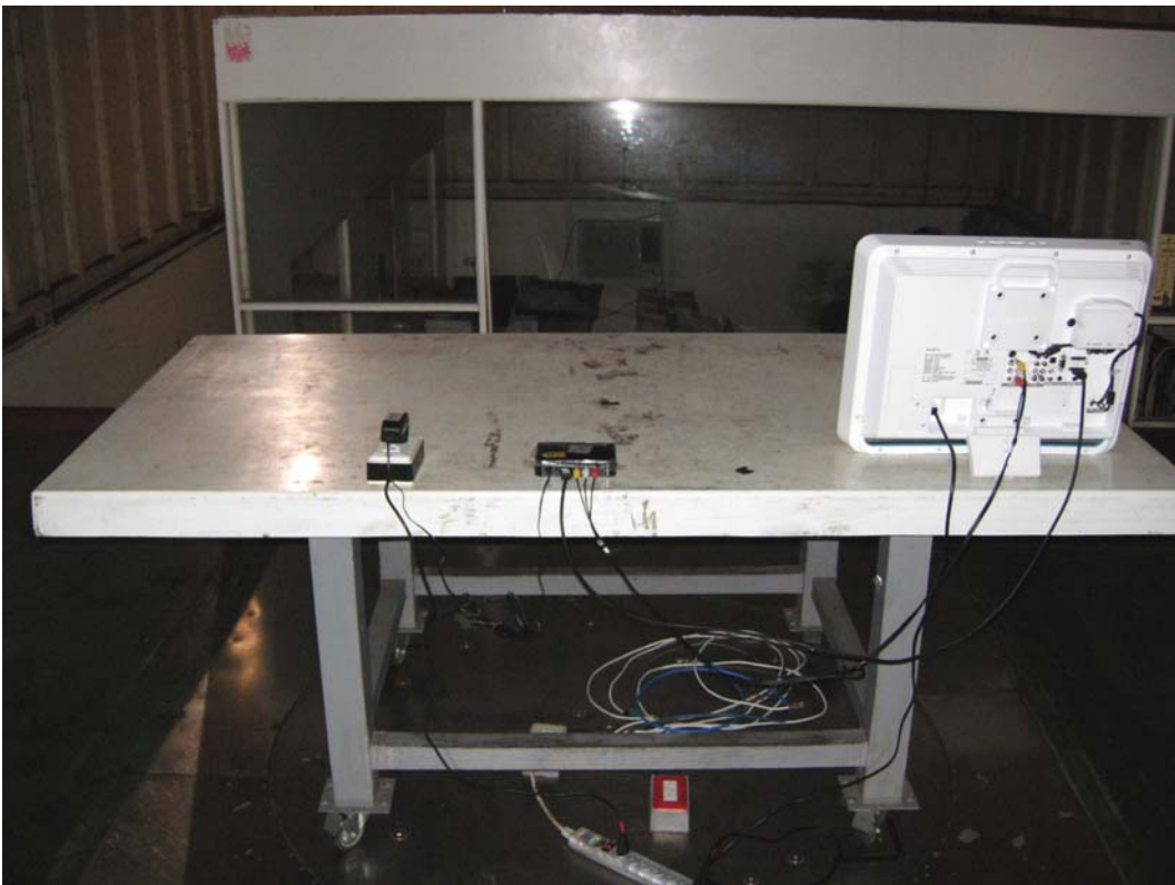
Back View of Radiated Test (Horn) 1-18GHz
