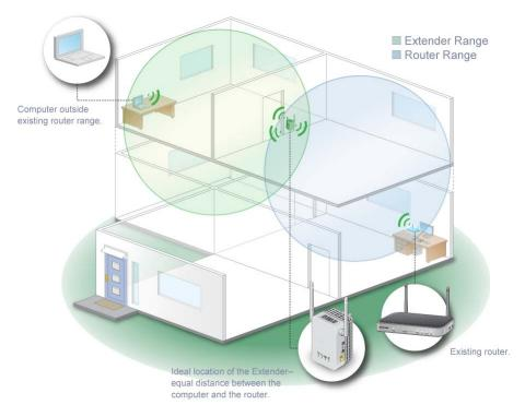
The range extender must do each of these jobs so that both ends of the bridge are in place.
