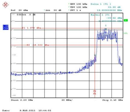
High Band Edge Plot on Configuration IEEE 802.11n MCS0 40MHz Ant. 1 + Ant. 2 / 2452 MHz
