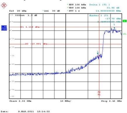
High Band Edge Plot on Configuration IEEE 802.11g Ant. 1 / 2462 MHz
