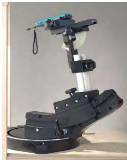
Fig. 6 Device holder supplied by SPEAG
