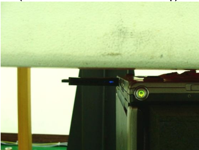
Direct Laptop Plug-in for USB Configuration 1 (for Back Off SAR) (Horizontal Up with Phantom 10 mm Gap)
