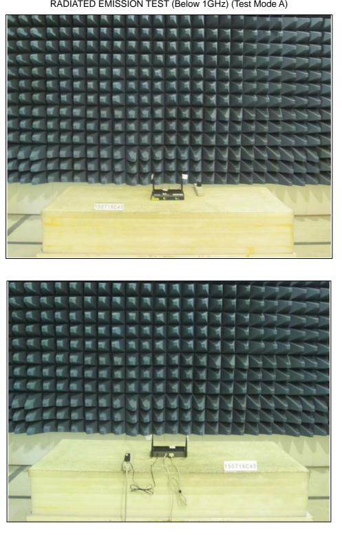
RADIATED EMISSION TEST (Below 1GHz) (Test Mode A)
