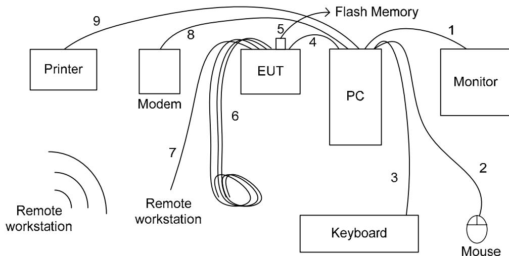
1. The VGA cable is connected from PC to Monitor.
