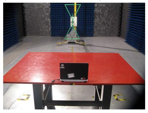
Test Mode: Mode 2: Transmit by 802.11gDescription: Front View of Radiated Emission Test Setup for Above 1GHz
