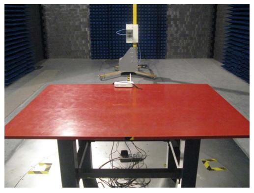
Test Mode: Mode 1: Transmit by 802.11bDescription: Back View of Radiated Emission Test Setup for Above 1GHz
