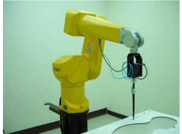
Fig. 5.2 Probe setup on robot
