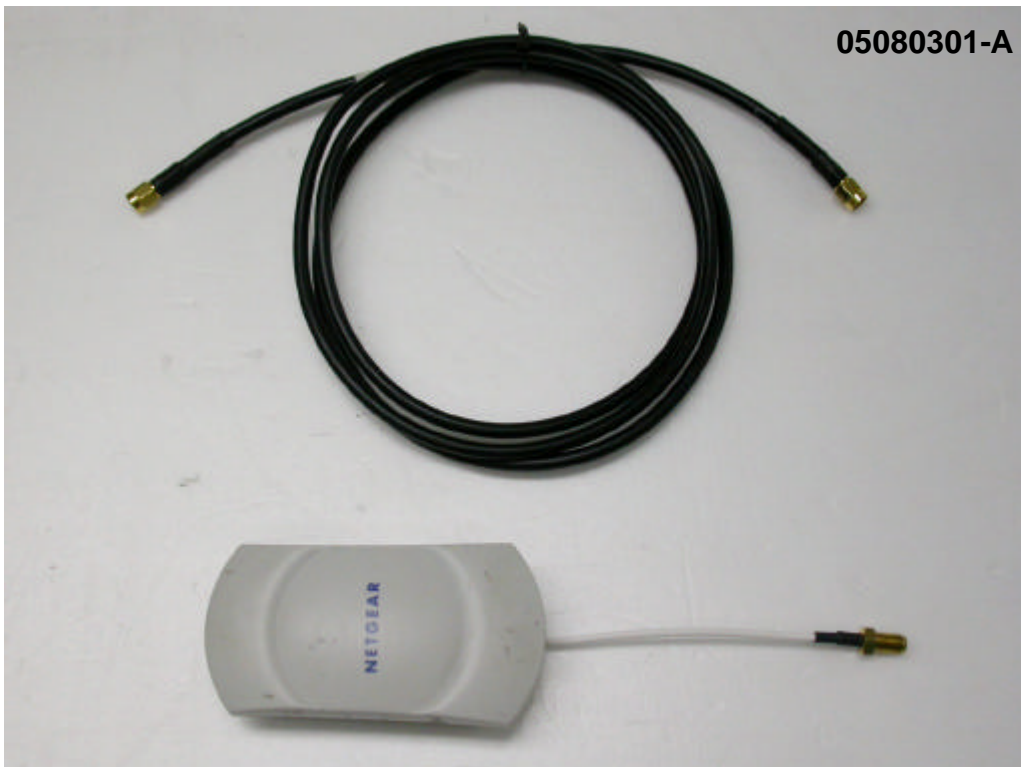
Ceiling antenna (Antenna gain 5dBi- ANT2405)
