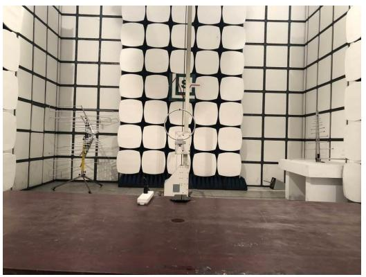
Radiated Emission below 30MHz-AC adapter charge mode
