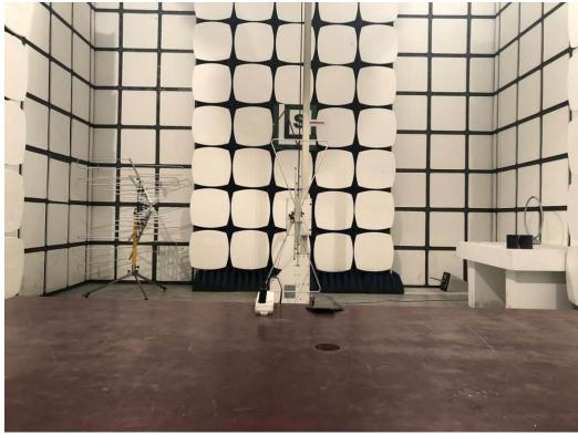
Radiated Emission below 1GHz-AC adapter charge mode
