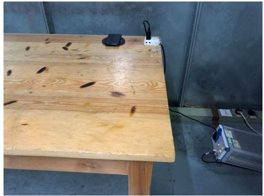
Conducted Emission-AC adapter charge mode
