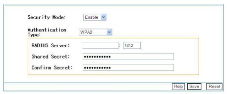
WPA 2 is the enhancement of WPA which uses the AES encryption algorithm.
