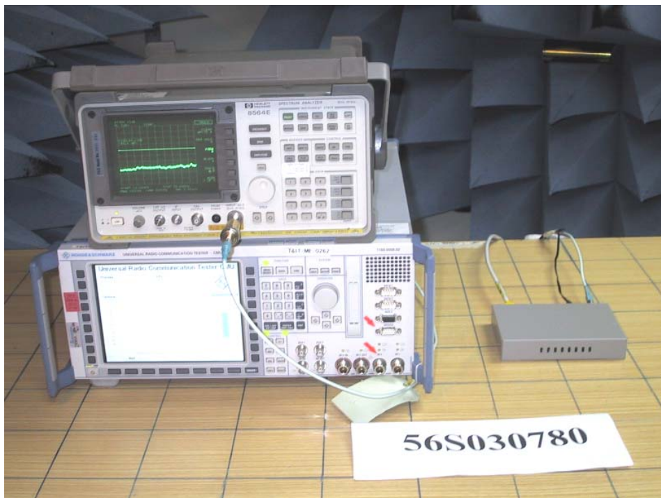
Peak Power Spectral Density Measurement Test Setup
