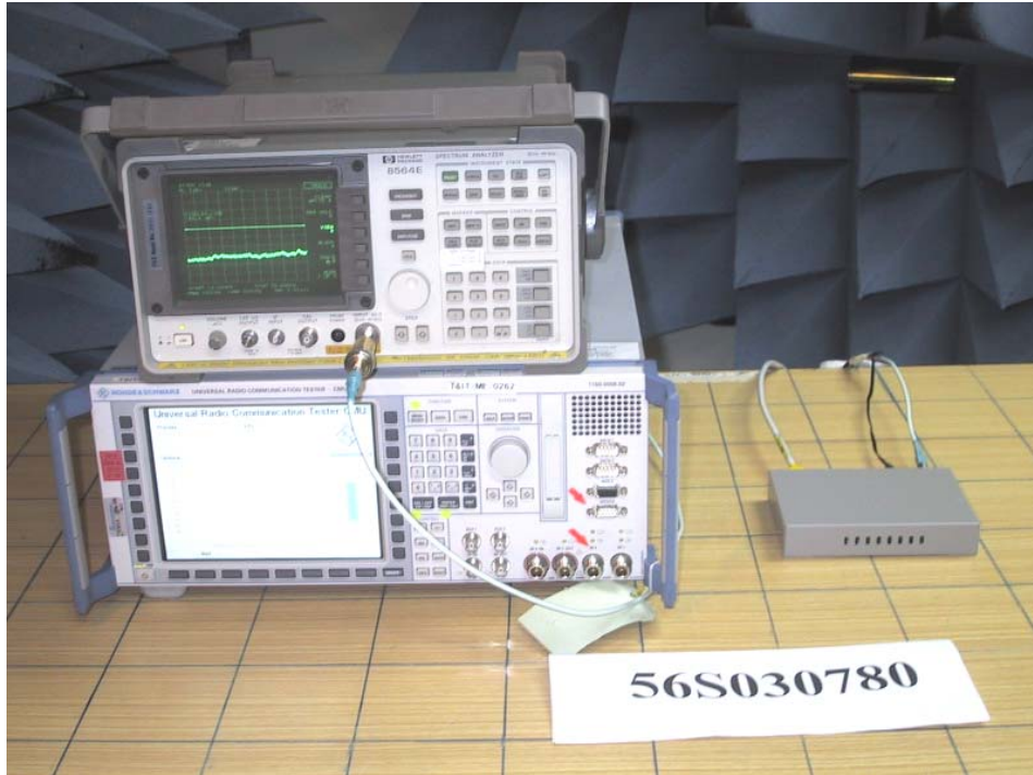
Spectrum Bandwidth Measurement Test Setup
