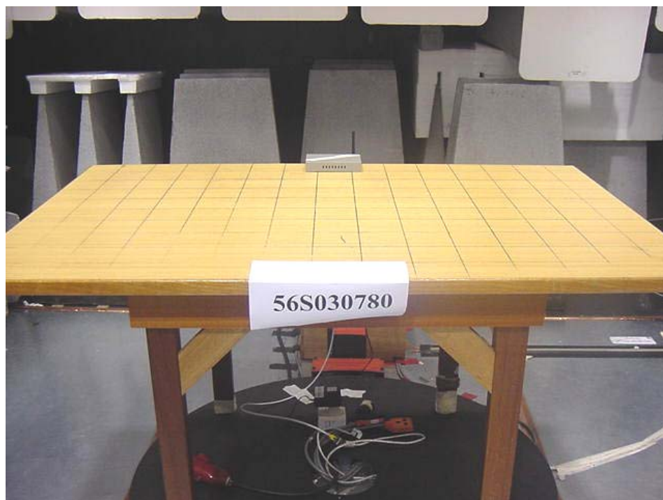
Radiated Emissions Setup (Front View)
