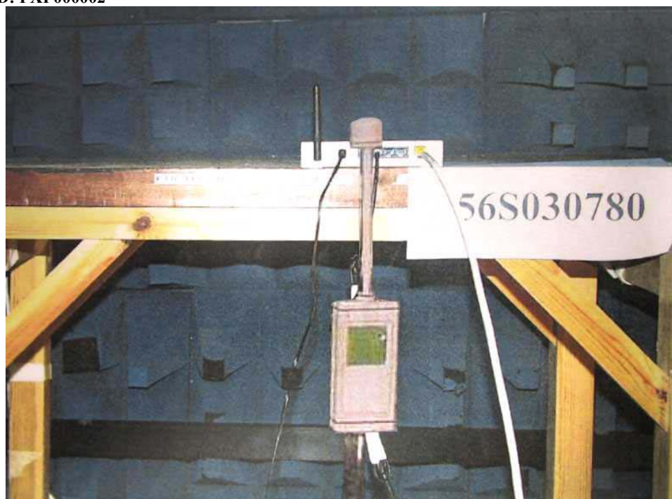
Maximum Permissible Exposure Measurement Test Setup
