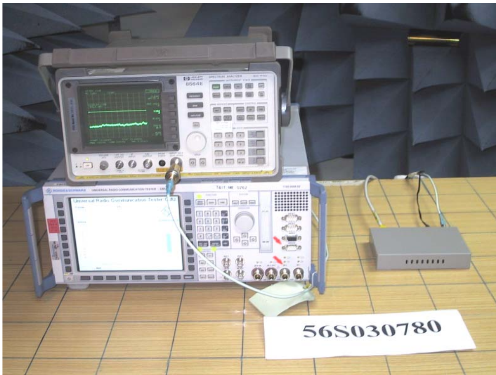
Peak Power Spectral Density Measurement Test Setup
