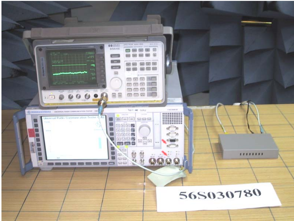
Spectrum Bandwidth Measurement Test Setup
