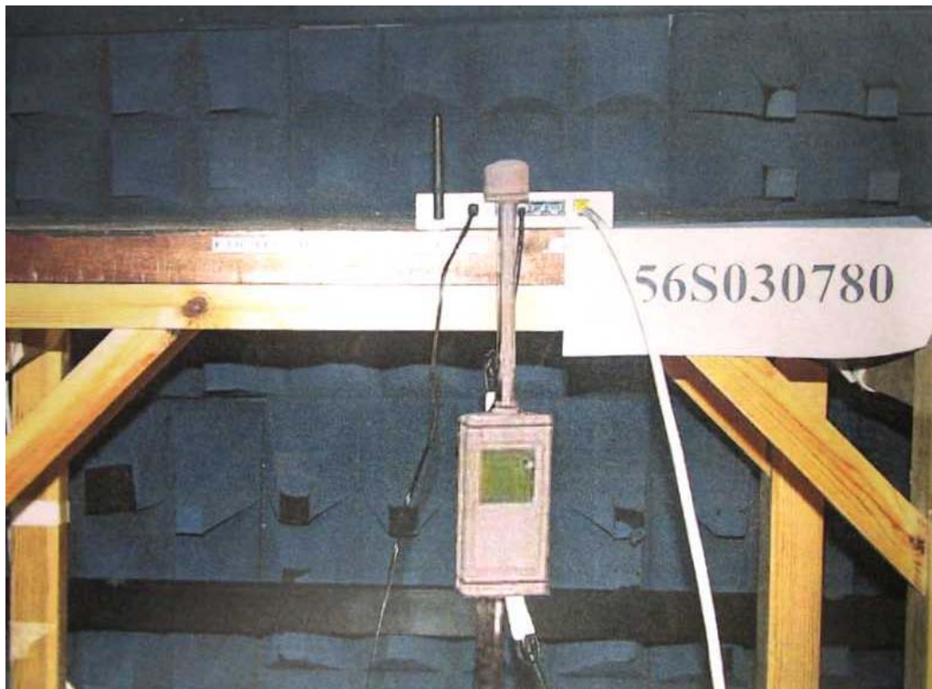
Maximum Permissible Exposure Measurement Test Setup
