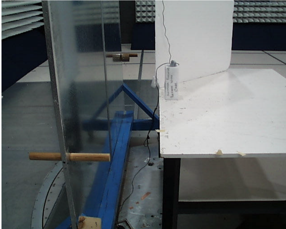
Figure 10-5: Configuration photograph, AC mains conducted emission, rear view
