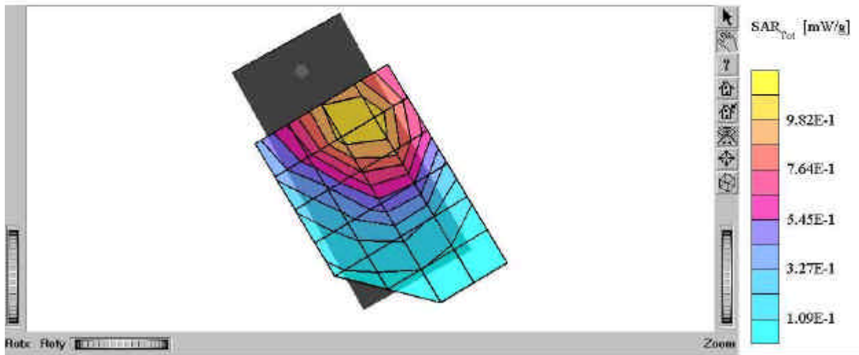
Distribution of maximum SAR in 835 AMPS band. Measured against the right hand side of the head in the “Cheek” position. Picture shows the bottom part of the phone.
