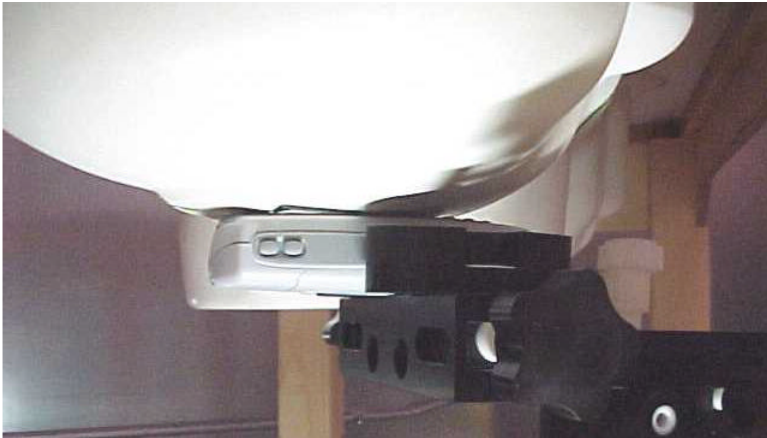
Position of device against head phantom using the “cheek” position
