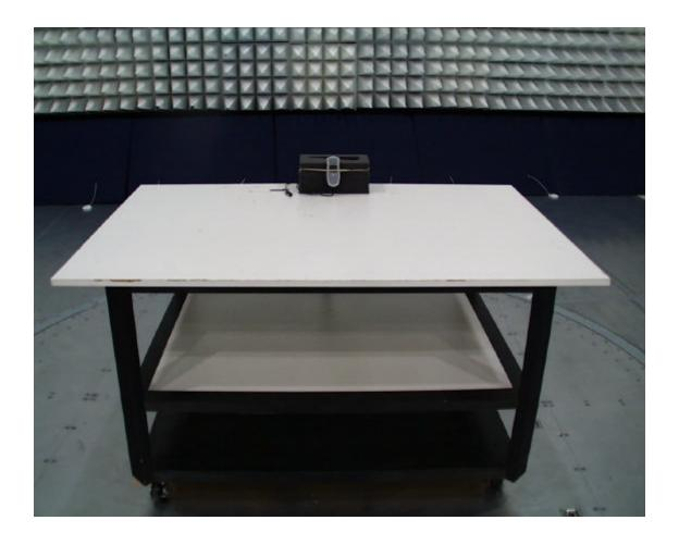
Figure 13.5-1: Configuration photograph, radiated emission, front view
