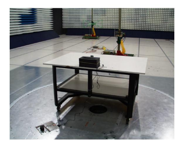
Figure 13.5-2: Configuration photograph, radiated emission, rear view
