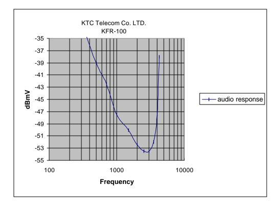
Applicant: KTC Telecom Co., Ltd. FCC ID: PXBKFR-100 Report #: T:\K\KTCTELE\913ZAK1\913ZAK1TestReport.doc Page #: 3 of 13 2.1047(b) <u>Audio\_input\_versus\_modulation</u> The audio input level needed for a particular perpercentage of modulation was measured in accordance with TIA/EIA Specification 603. The audio input curves versus modulation are shown in the following pages. Curves are provided for audio input frequencies of 300, 1000, and 3000 Hz.
