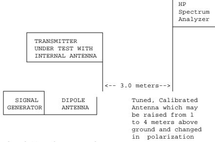
Equipment placed 80cm above ground on a rotatable platform.
