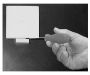
If you need to remove the repeater please separate it from the suspension holder with a gentle push of a screwdriver.
