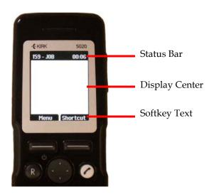
The display is divided in three parts: **Status bar**, **Display center** and **Softkey Text** (see figure above).
