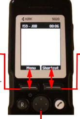
Right Softkey Pressing right softkey activates right softkey text.
