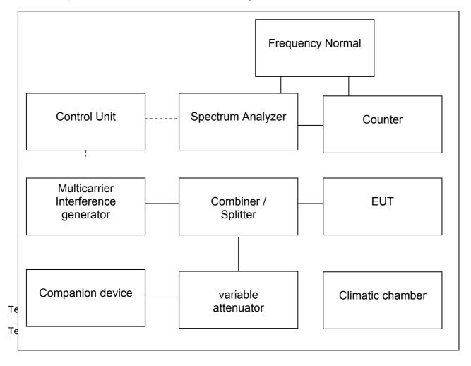
Monitoring tests generally determine the lower and upper threshold of the EUT , and verify that if the EUT is operating in the "least-interfered channel" mode, it can properly select the channel with the lowest interference power, within a 6 dB resolution. The "preferred" end of the 1920-1930 MHz band denotes the
