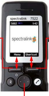
Right Softkey Pressing right softkey activates right softkey text.
