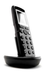
For correct charging, be sure the room temperature is between 0°C/32°F and 40°C/104°F. Do not place the handset in direct sunlight. The battery has a built-in heat sensor which will stop charging if the battery temperature is too high.
