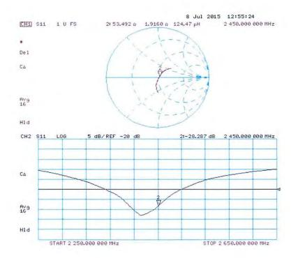
Impedance Measurement Plot for Head TSL
