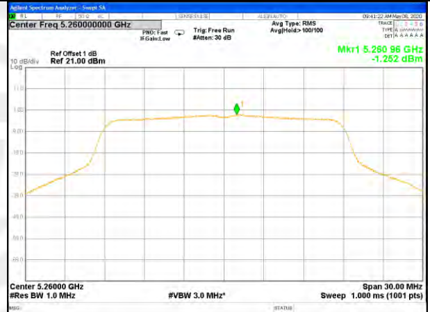
W53_11n20_Higher_Power Spectrum Density
