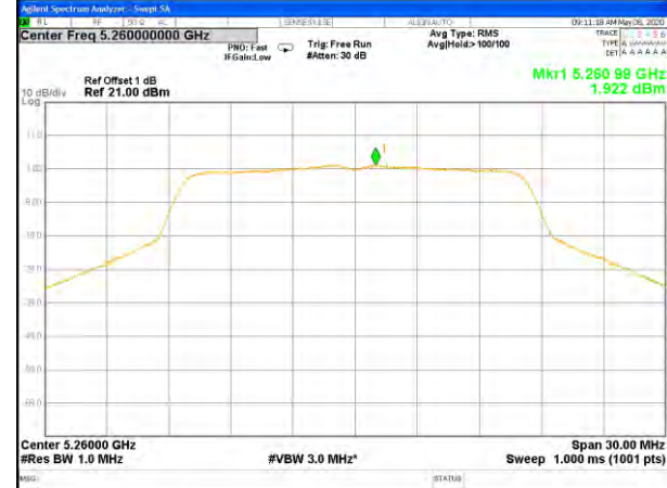
W53_11a20_Higher_Power Spectrum Density
