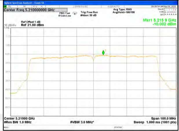
W52_11ac80_CH42(5210MHz)_Power Spectrum Density
