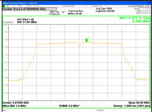
W56_11ac80_Higher_Power Spectrum Density
