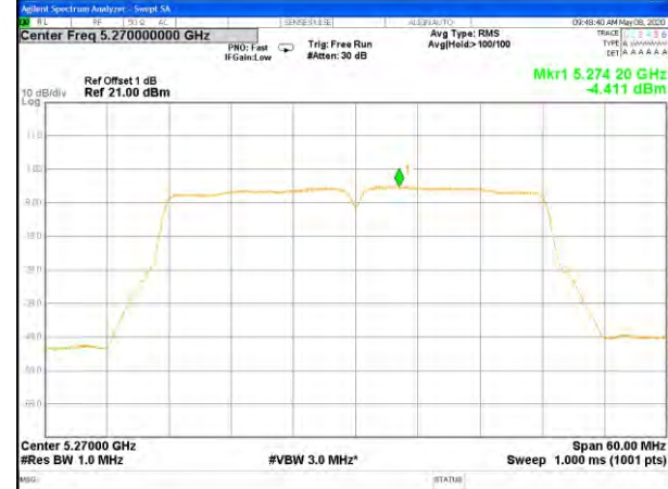
W53_11ac20_Lower_Power Spectrum Density
