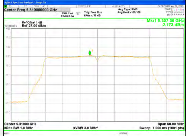
W53_11ac20_Middle_Power Spectrum Density
