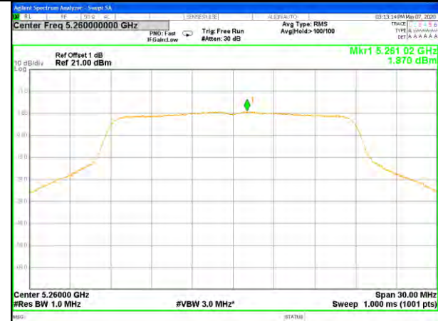
W53_11ac20_Higher_Power Spectrum Density
