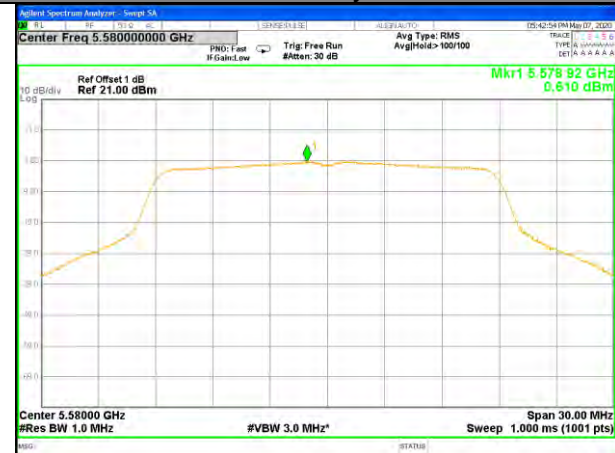
W56_11ac20_Middle_Power Spectrum Density
