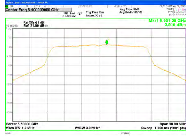
W56_11a20_Higher_Power Spectrum Density
