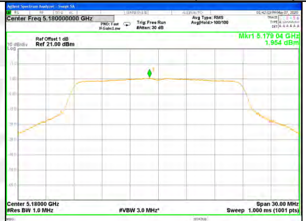
W52_11n20_Higher_Power Spectrum Density
