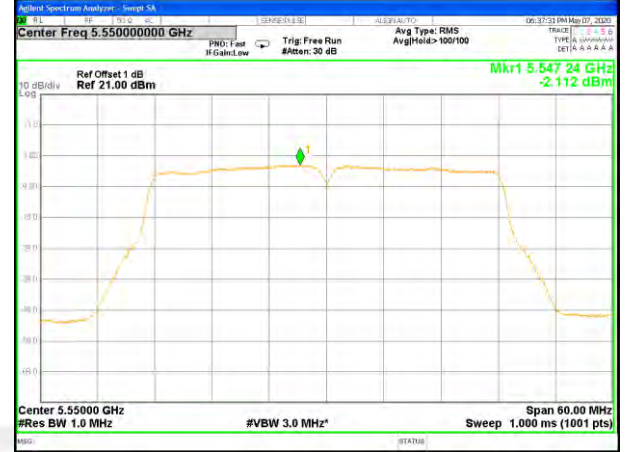
W56_11ac80_Lower_Power Spectrum Density
