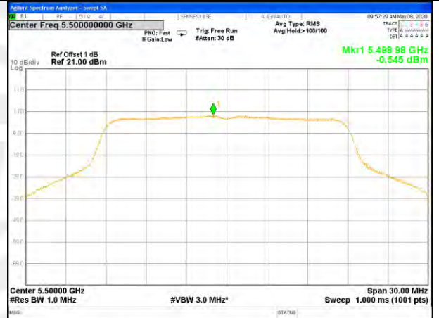
W56_11n20_Higher_Power Spectrum Density
