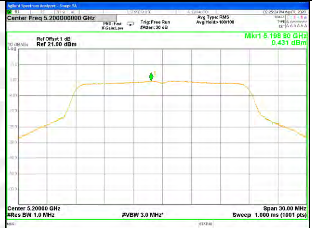
W52_11ac40_Lower_Power Spectrum Density
