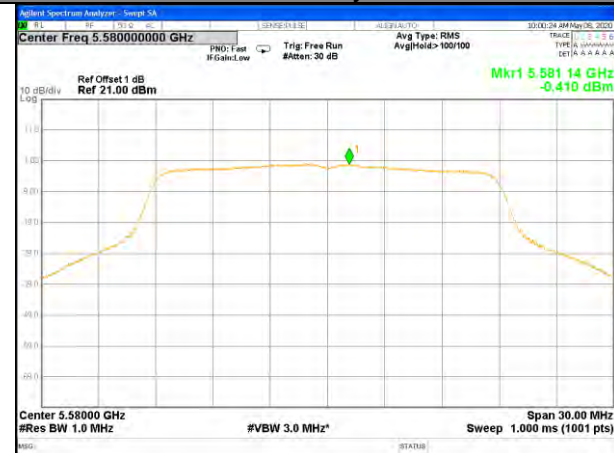
W56_11ac20_Middle_Power Spectrum Density
