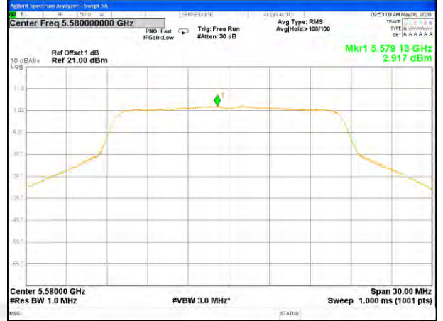
W56_11n20_Lower_Power Spectrum Density
