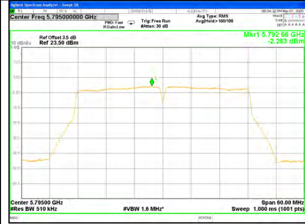
W58_11ac40_Higher_Power Spectrum Density
