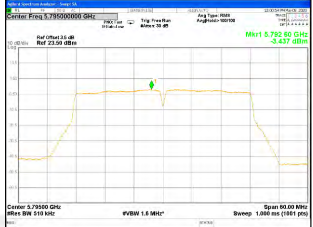
W58_11ac20_Middle_Power Spectrum Density
