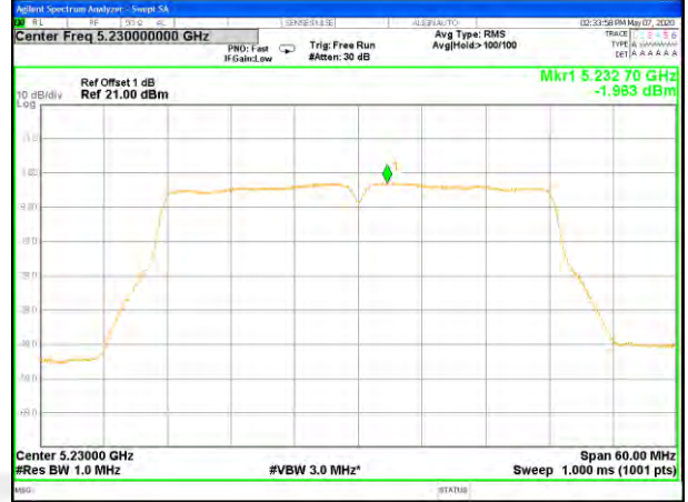
W52_11ac20_Middle_Power Spectrum Density
