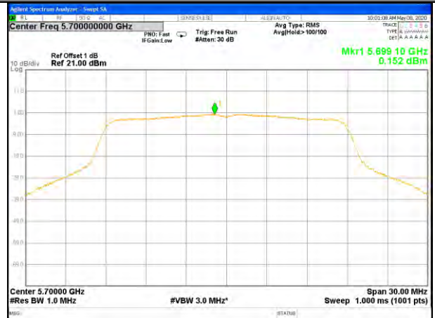
W56_11ac20_Higher_Power Spectrum Density
