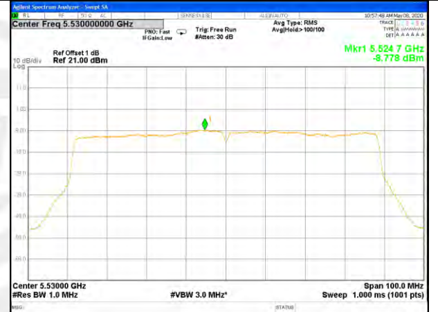
W56_11ac80_Lower_Power Spectrum Density
