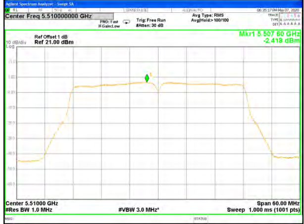
W56_11ac40_Higher_Power Spectrum Density
