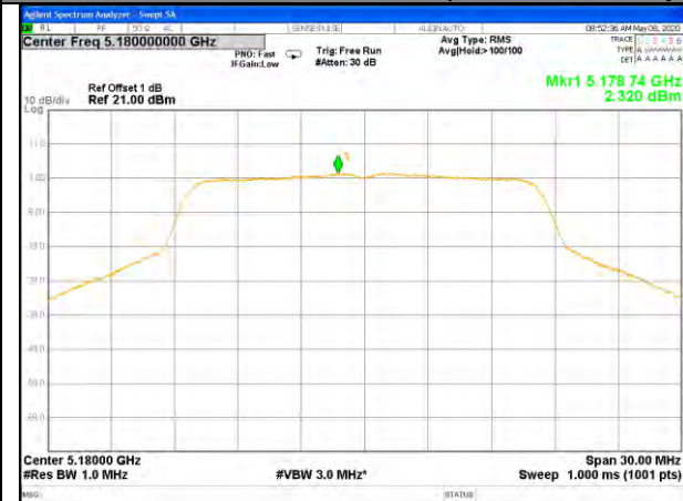
W52_11a20_Higher_Power Spectrum Density
