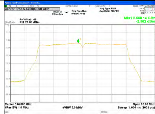
W56_11ac20_Middle_Power Spectrum Density
