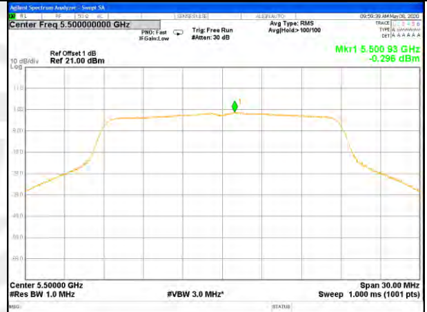
W56_11ac20_Higher_Power Spectrum Density
