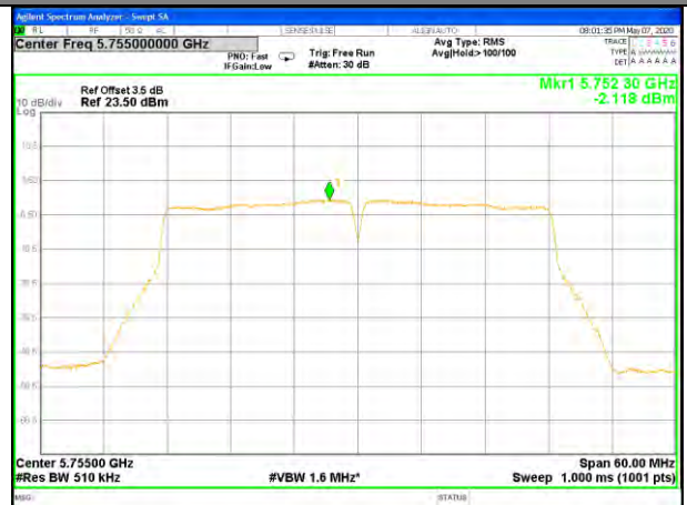
W58_11ac40_Lower_Power Spectrum Density
