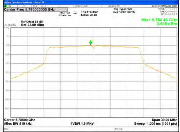
W58_11n20_Lower_Power Spectrum Density
