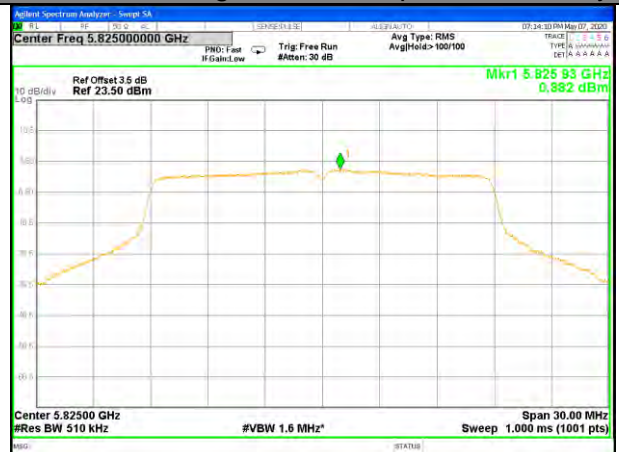
W58_11n20_Higher_Power Spectrum Density
