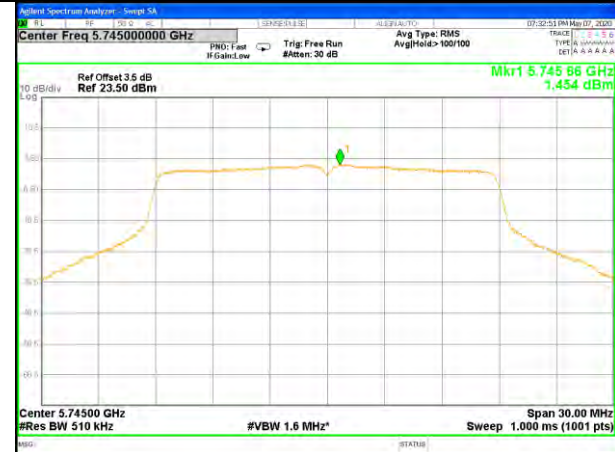
W58_11ac20_Higher_Power Spectrum Density
