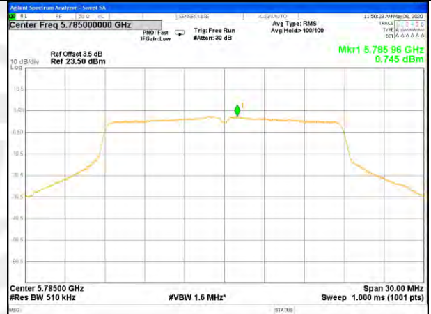
W58_11ac40_Lower_Power Spectrum Density
