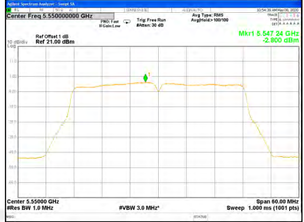
W56_11ac20_Lower_Power Spectrum Density
