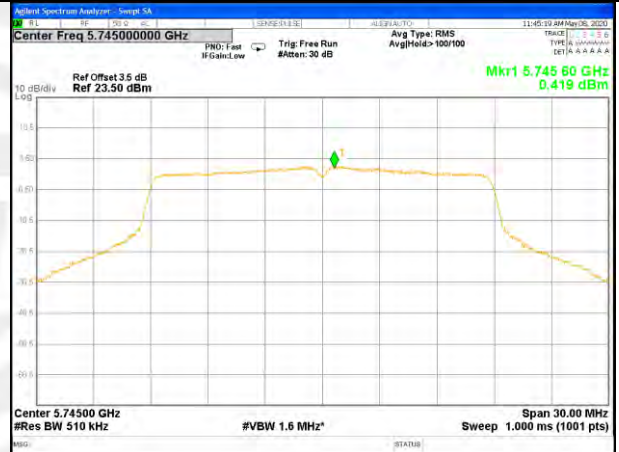
W58_11n20_Higher_Power Spectrum Density
