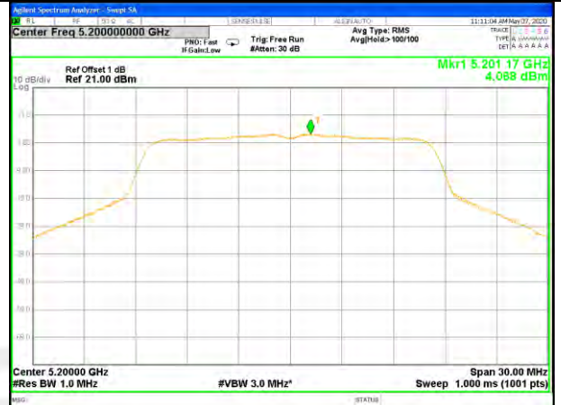
W52_11n20_Lower_Power Spectrum Density
