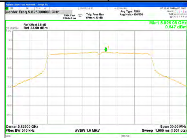
W58_11ac20_Higher_Power Spectrum Density
