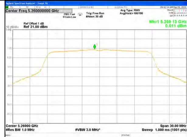
W53_11ac20_Higher_Power Spectrum Density
