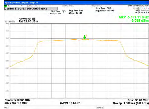
W52_11ac20_Higher_Power Spectrum Density
