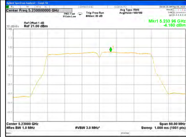
W52_11ac40_Higher_Power Spectrum Density
