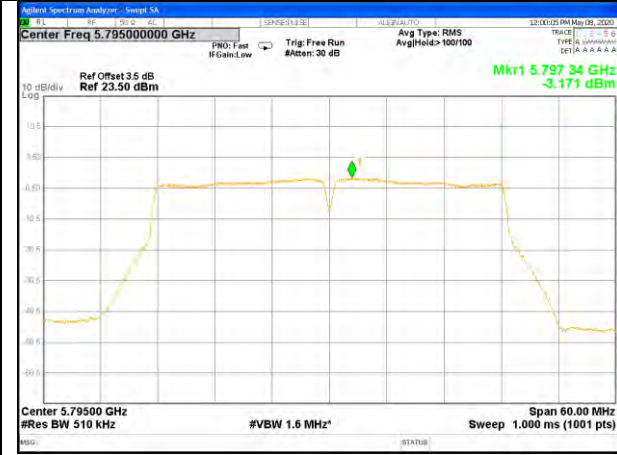
W58_11ac40_Higher_Power Spectrum Density
