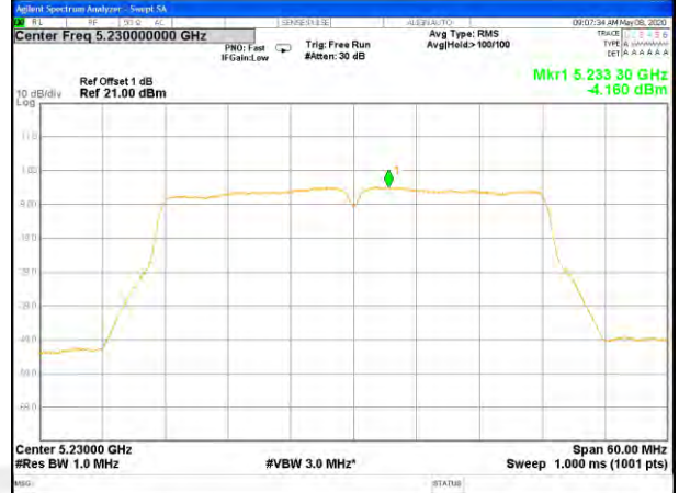
W52_11ac20_Middle_Power Spectrum Density
