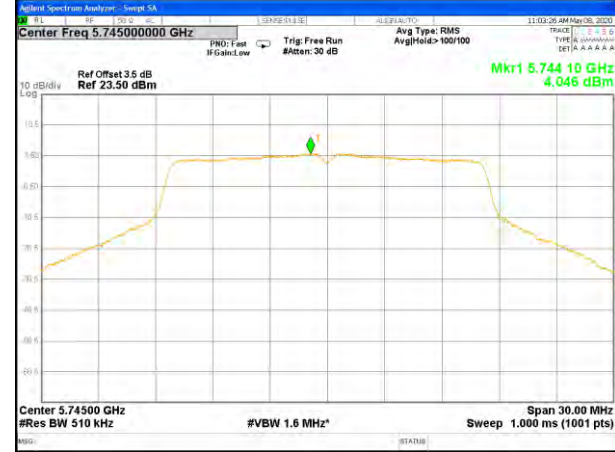
W58_11a20_Higher_Power Spectrum Density
