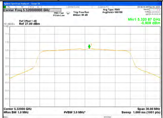
W53_11n20_Higher_Power Spectrum Density
