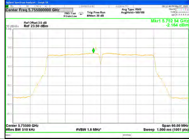
W58_11ac20_Lower_Power Spectrum Density
