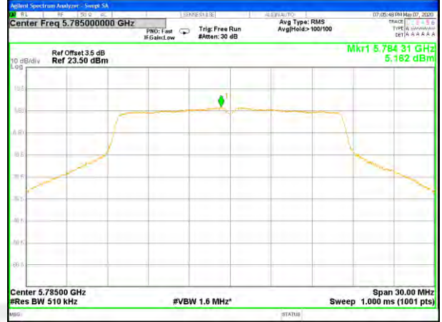
W58_11n20_Lower_Power Spectrum Density
