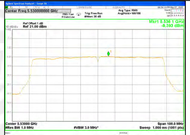
W56_11ac80_Lower_Power Spectrum Density
