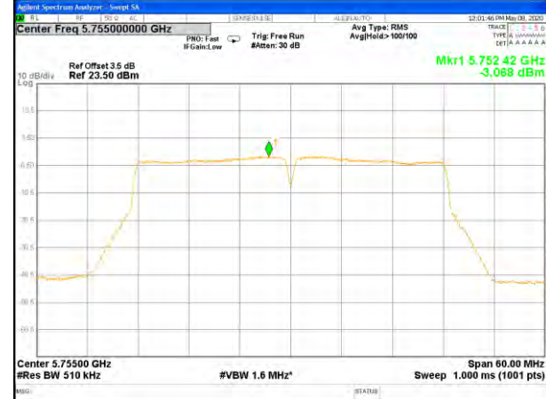
W58_11ac20_Lower_Power Spectrum Density
