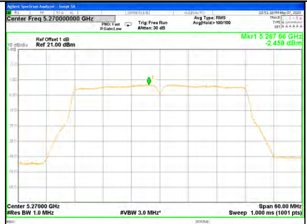
W53_11ac40_Lower_Power Spectrum Density
