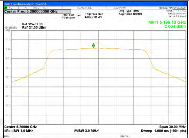
W52_11n20_Lower_Power Spectrum Density
