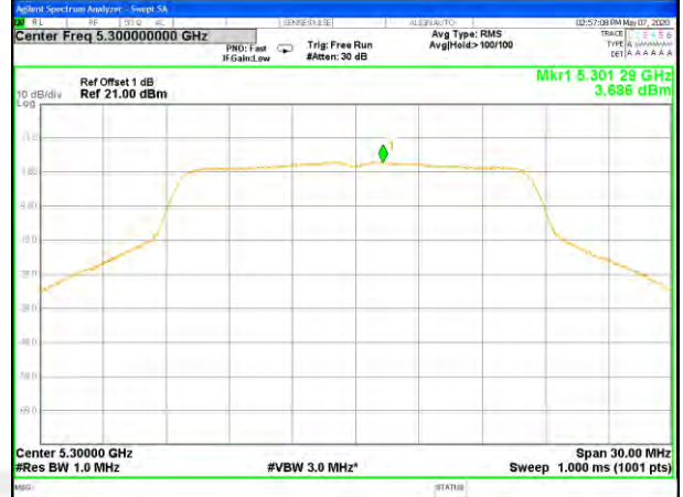
W53_11n20_Lower_Power Spectrum Density
