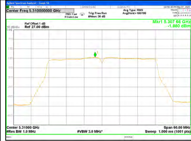
W53_11ac40_Higher_Power Spectrum Density
