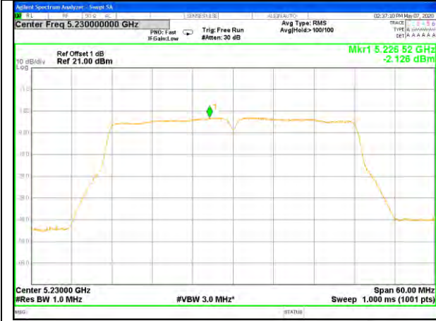
W52_11ac40_Higher_Power Spectrum Density
