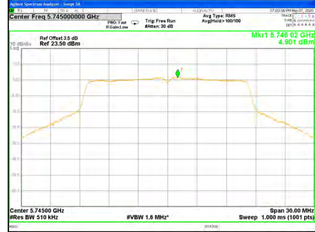
W58_11a20_Higher_Power Spectrum Density
