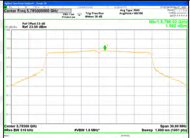
W58_11ac40_Lower_Power Spectrum Density
