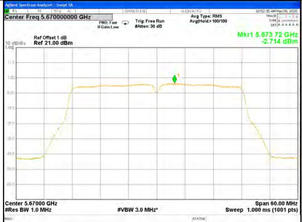
W56_11ac80_Higher_Power Spectrum Density
