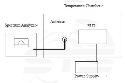
The EUT which is powered by the Battery, is coupled to the Spectrum Analyzer; the RF load attached to the EUT antenna terminal is 500hm; the path loss as the factor is calibrated to correct the reading.
