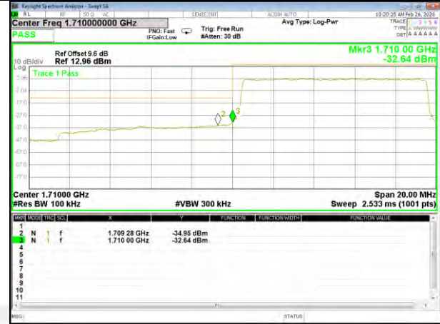
QPSK_10M_Higher_Band edge_Full-RB
