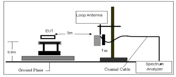
(B) Radiated Emission Test-Up Frequency 30MHz~1GHz
