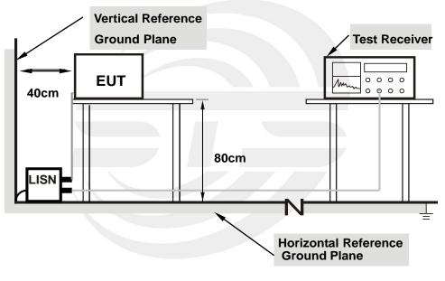
Note: 1.Support units were connected to second LISN. 2.Both of LISNs (AMN) are 80 cm from EUT and at least 80 cm from other units and other metal planes support.
