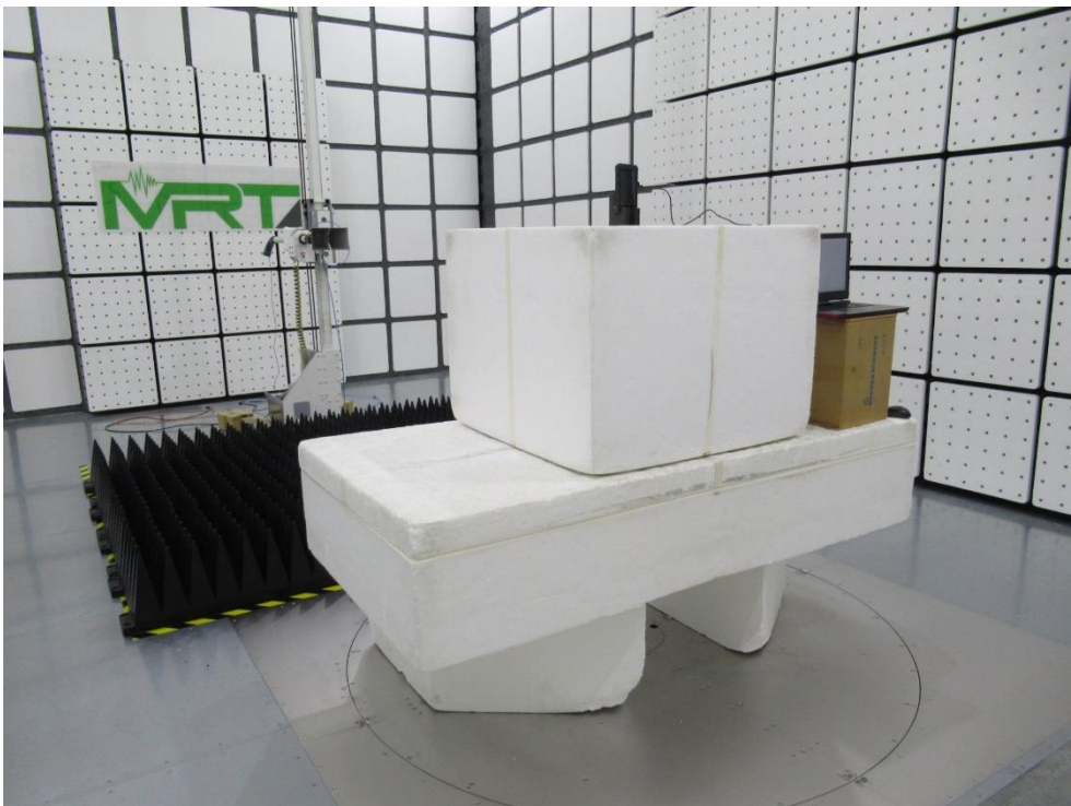
Description: Radiated Emission Test Setup for 1GHz~18GHz
