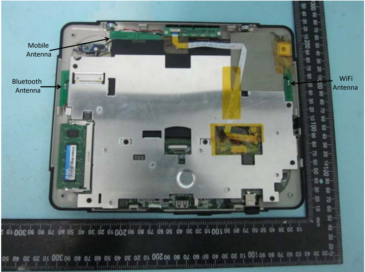
Transmit Antenna Location
