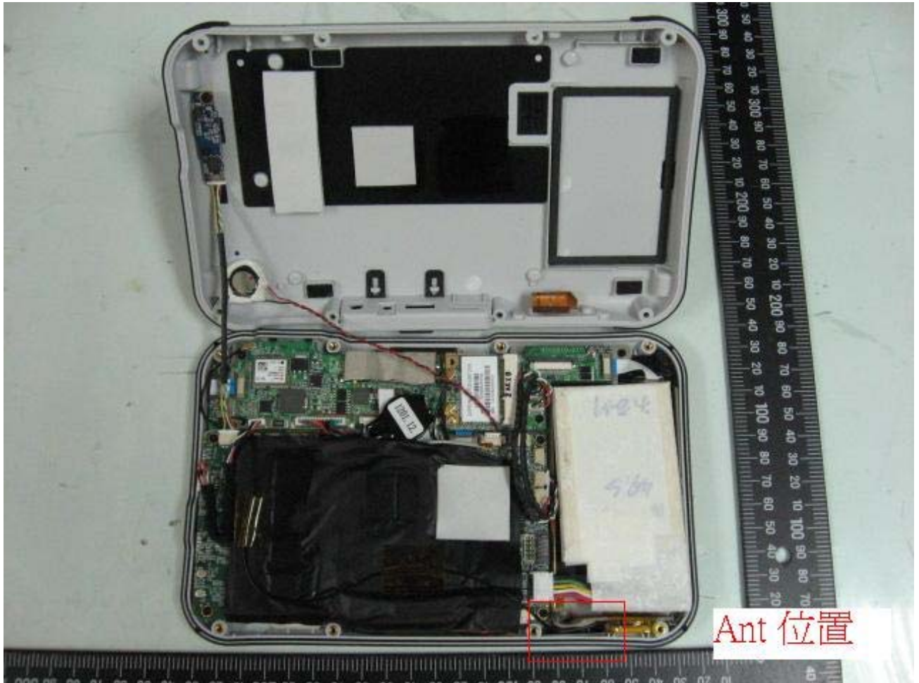
EUT inside View and Transmit Antenna Location
