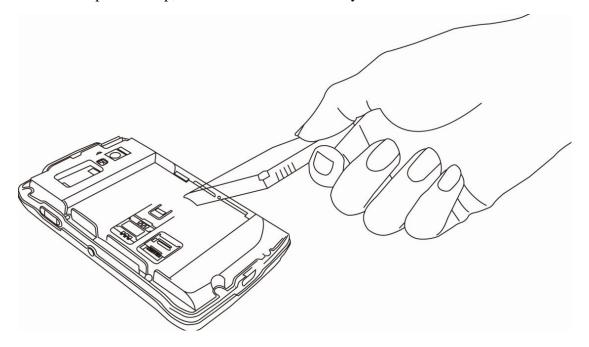
4. Push the metal cover backward and lift the metal cover. Then put the SD card into the socket, close the metal cover and push forward till click sound.
