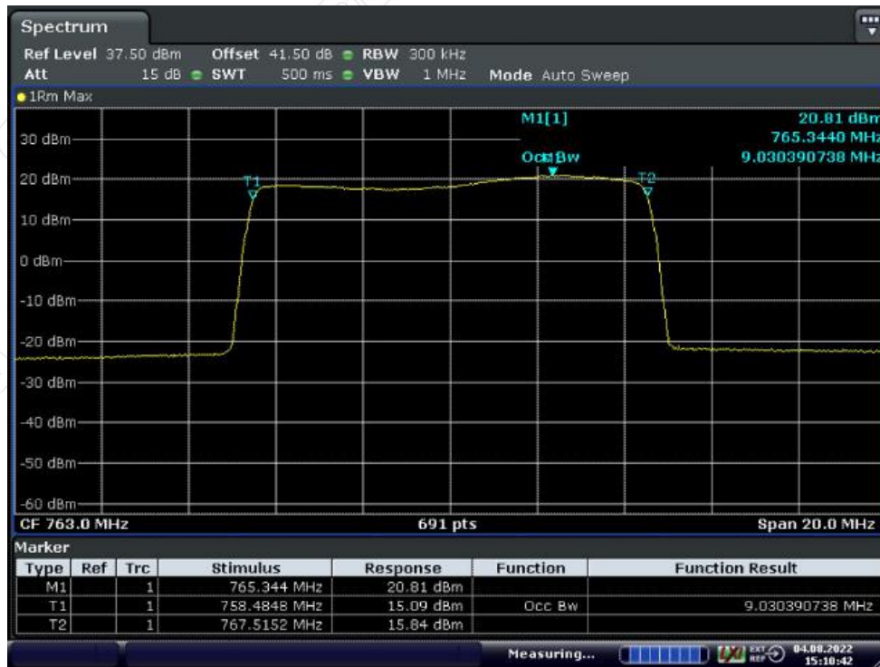
Middle Frequency: 763.0MHz, Output occupied BW (with the input signal amplitude set 3 dB above the AGC threshold)
