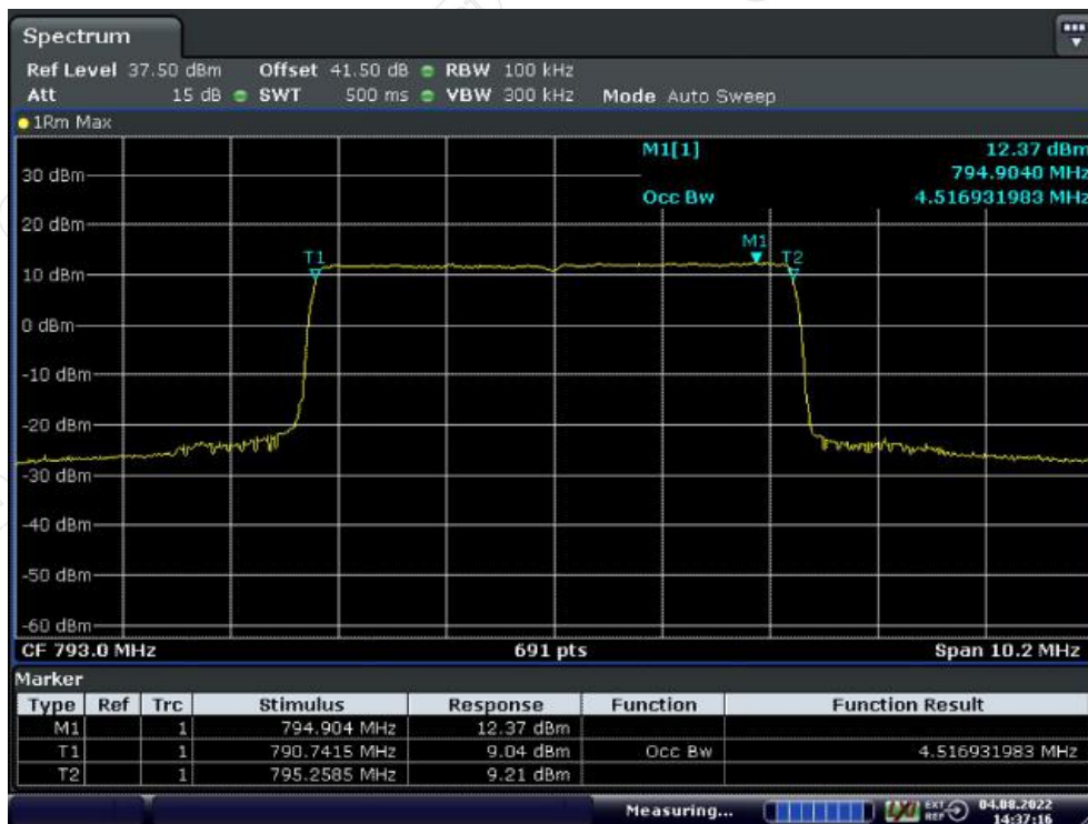
Middle Frequency: 793.0MHz, Output occupied BW (with the input signal amplitude set 3 dB above the AGC threshold)
