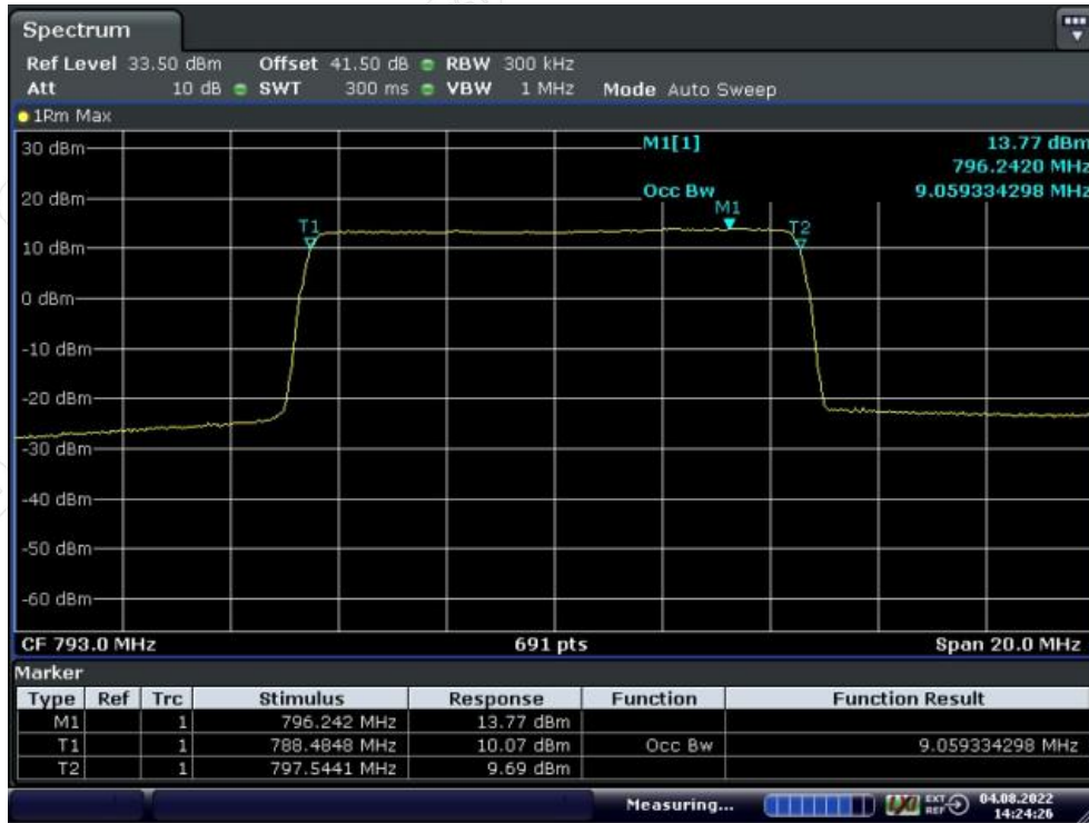
Middle Frequency: 793.0MHz, Output occupied BW(AGC)
