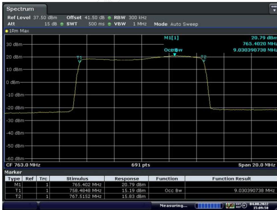
Middle Frequency: 763.0MHz, Output occupied BW(AGC)
