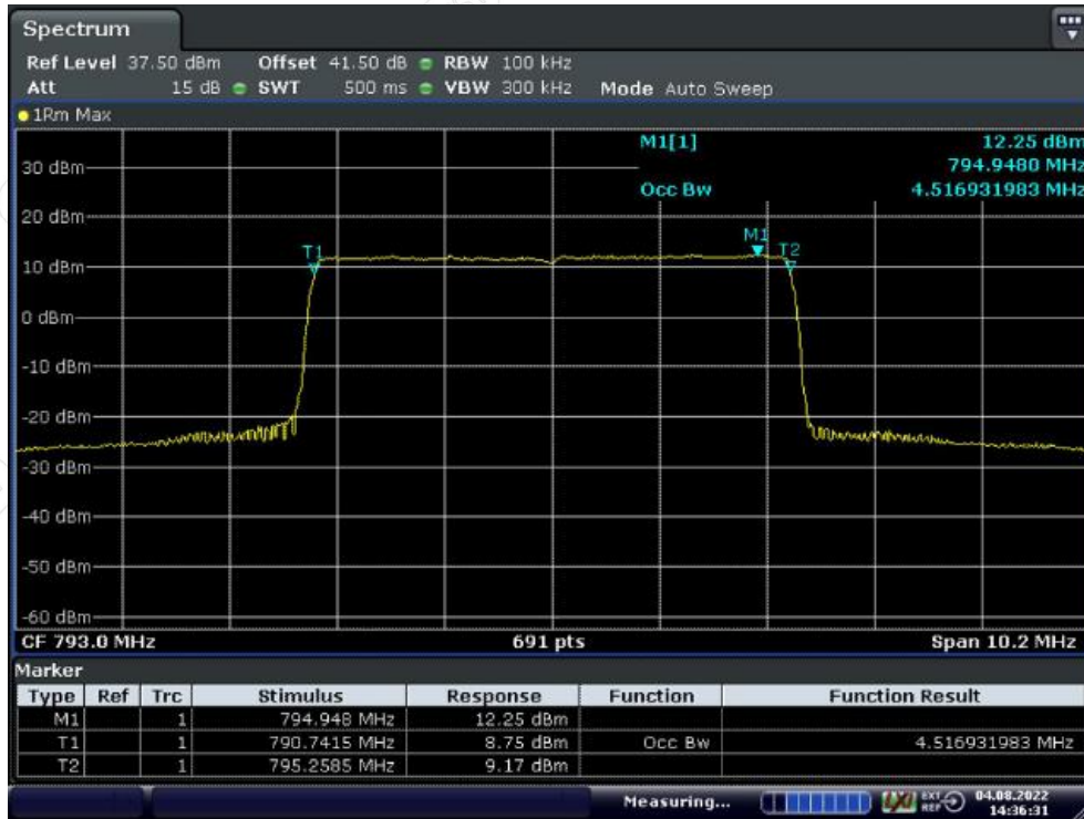
Middle Frequency: 793.0MHz, Output occupied BW(AGC)
