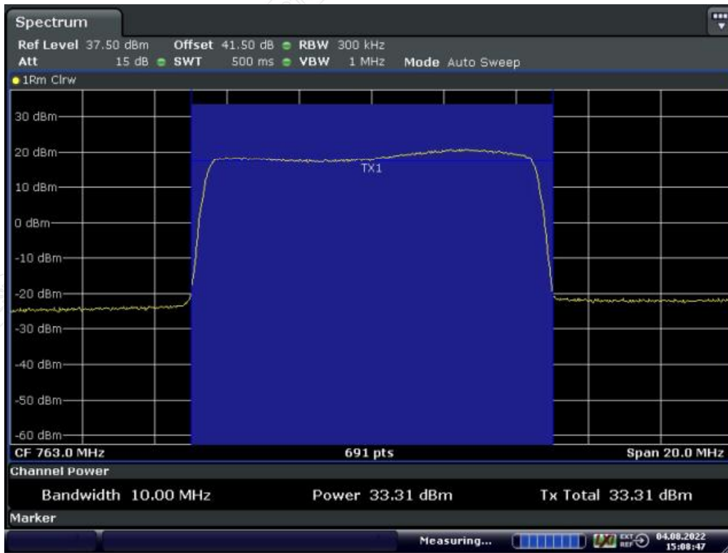
Middle Frequency: 763.0MHz, Output occupied BW(AGC)
