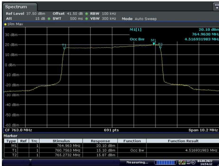
Middle Frequency: 763.0MHz, Output occupied BW(AGC)
