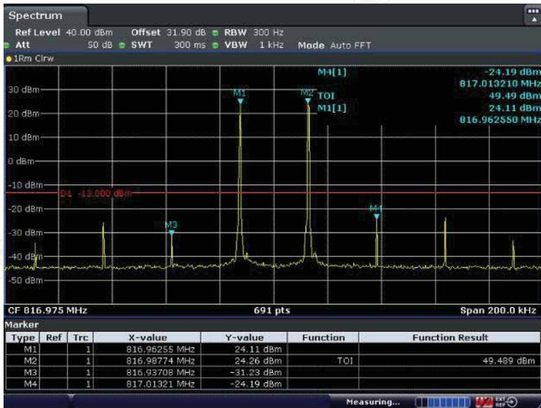
High Frequency and with the input signal amplitude set 3 dB above the ALC threshold
