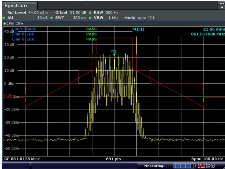
With the input signal amplitude set the AGC threshold Lowest Frequency: 861.0125MHz
