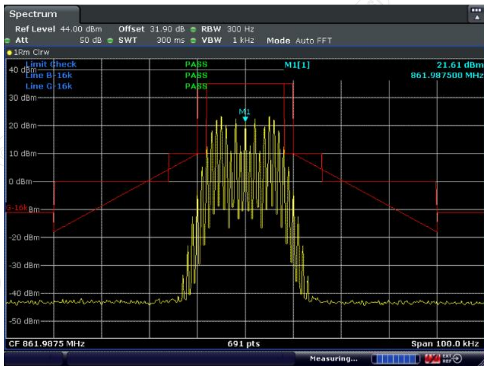
With the input signal amplitude set 3 dB above the AGC threshold Highest Frequency: 861.9875MHz
